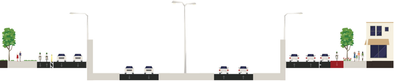
Figure 7. Woodward Avenue Cross Section between Poplar Park Boulevard and Elm Park Boulevard
